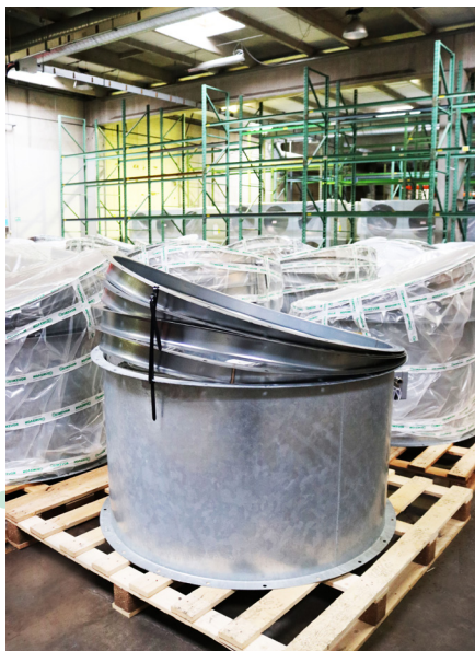
High temperature NovAx™ axial fans type ACN-1250 for ventilation and smoke exhaust in case of a fire
