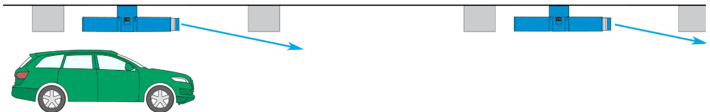
FIGURE 5B. JET FANS POSITIONED BETWEEN GIRDERS
