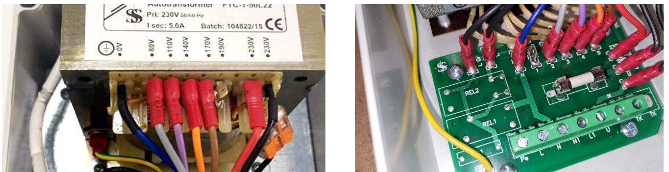
Figure 18. NV515 – 5-step regulator, minimum fan speed enabled (left) and location of N1 and L1 connectors (right)
